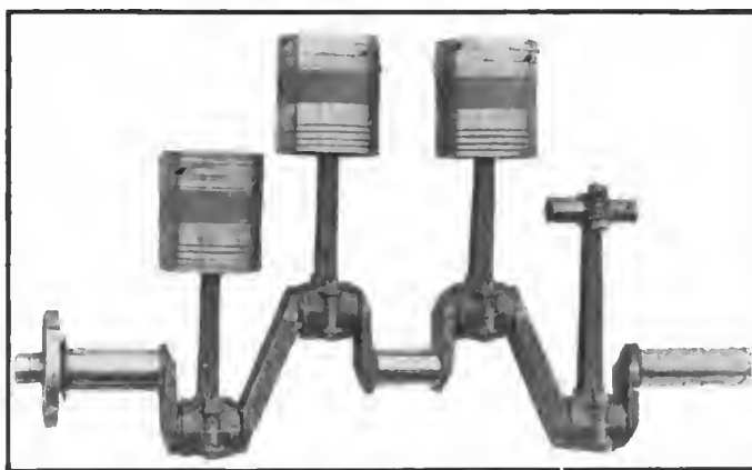
Fig. 4—The crankshaft with the connecting rods and pistons in place, showing a flanging for the flywheel and other refinements
